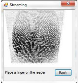
While the reader is in streaming mode, you can capture repeatedly by pressing a finger to the scanner plate. Click on the **Back** button to return to the main screen.
