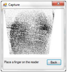
While the reader is in capture mode, you can capture repeatedly by pressing a finger to the scanner plate. Click on the **Back** button to return to the main screen.
